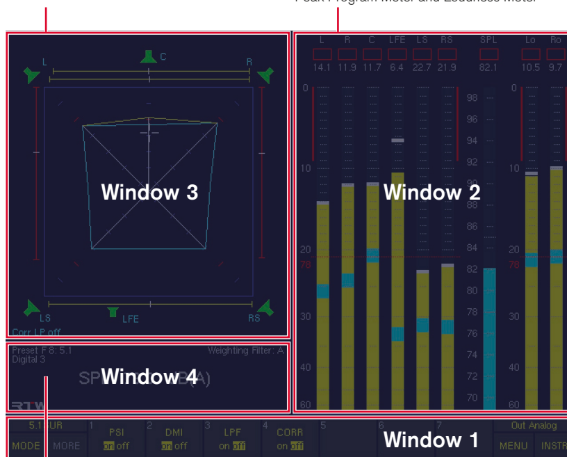
Window 2: Program Meter: Peak Program Meter and Loudness Meter
