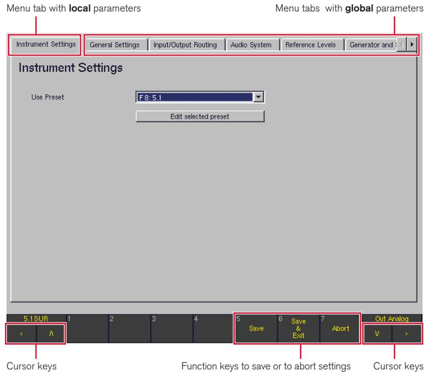
The menu system accesses all **local** parameters stored in presets as well as **global** settings that remain unchanged even after loading new presets.
