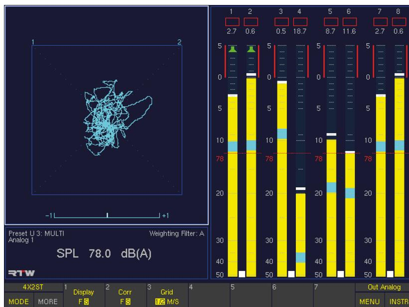
In Multi-Channel modes, the **VSC** input always follows the selected **Listening Group** provided it's a Stereo channel pair (bargraph pair with spot correlator and green loudspeaker symbols in the PPM).
