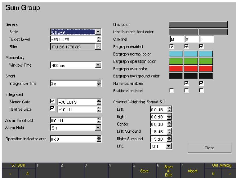
The **Sum Group**, located to the right of the channel bargraphs in the **Program Meter** display, contains up to three bargraphs showing the summed loudness of all channels in the Channel Group:
