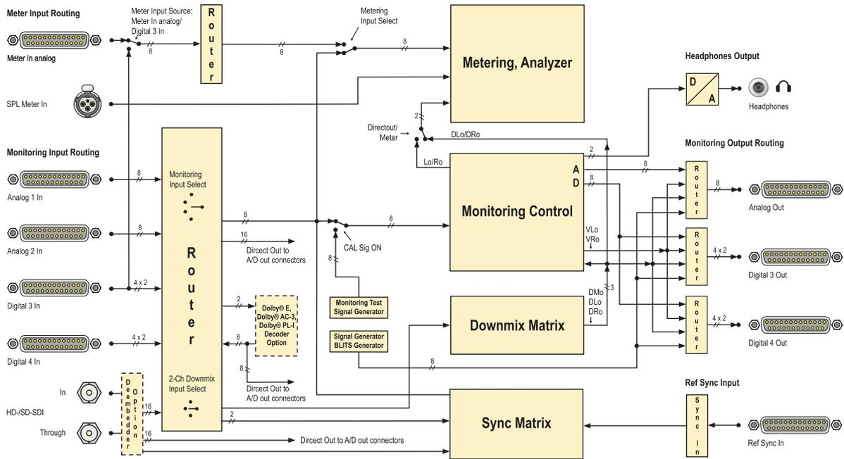
Internally, the unit uses logical channels (L, R, etc.) that match the selected audio format. For example, if you are using 5.1 surround, the internal logical channels are L, R, C, LS, RS, LFE, Lext, Rext, Lo and Ro. The assignment of the physical signal inputs to these logical channels is performed in the input routing, with separate settings for each input.
