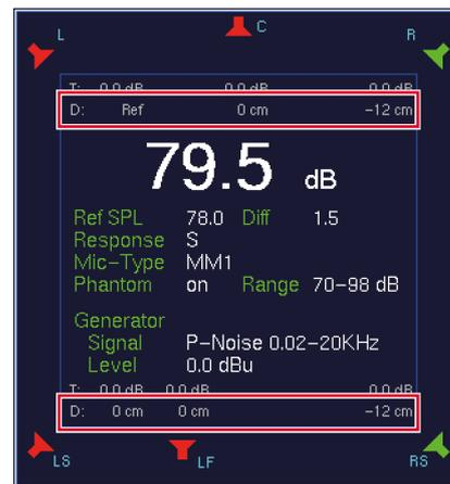
Example for **negative** Delay values in CAL instrument (above) and menu (below)
