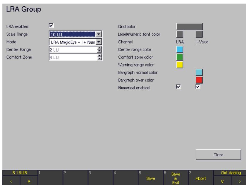
The **LRA Group**, located in the rightmost position of the **Program Meter** display, contains the **LRA** instrument. It displays a graphical representation of the loudness variances within short time periods. These are measured against the Loudness Range (LRA) descriptor specified in EBU R128. Also, the in-
