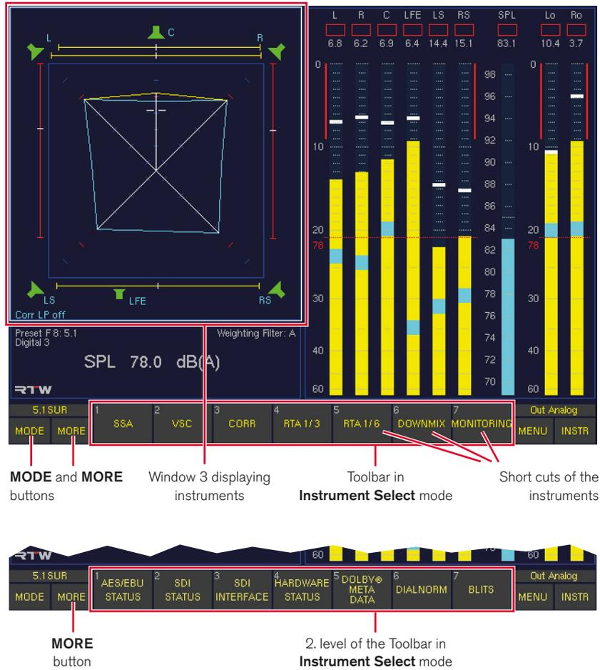
Window 3 (the top left area of the display) can show several instrument types (display modes), e. g. Surround Sound Analyzer (SSA), Vectorscope (VSC), Correlator (CORR) or RTA. Using the Instrument Select mode the instruments can be switched easily without loading new presets or accessing the menu system. Depending on the version of your unit up to 14 instruments are provided.
