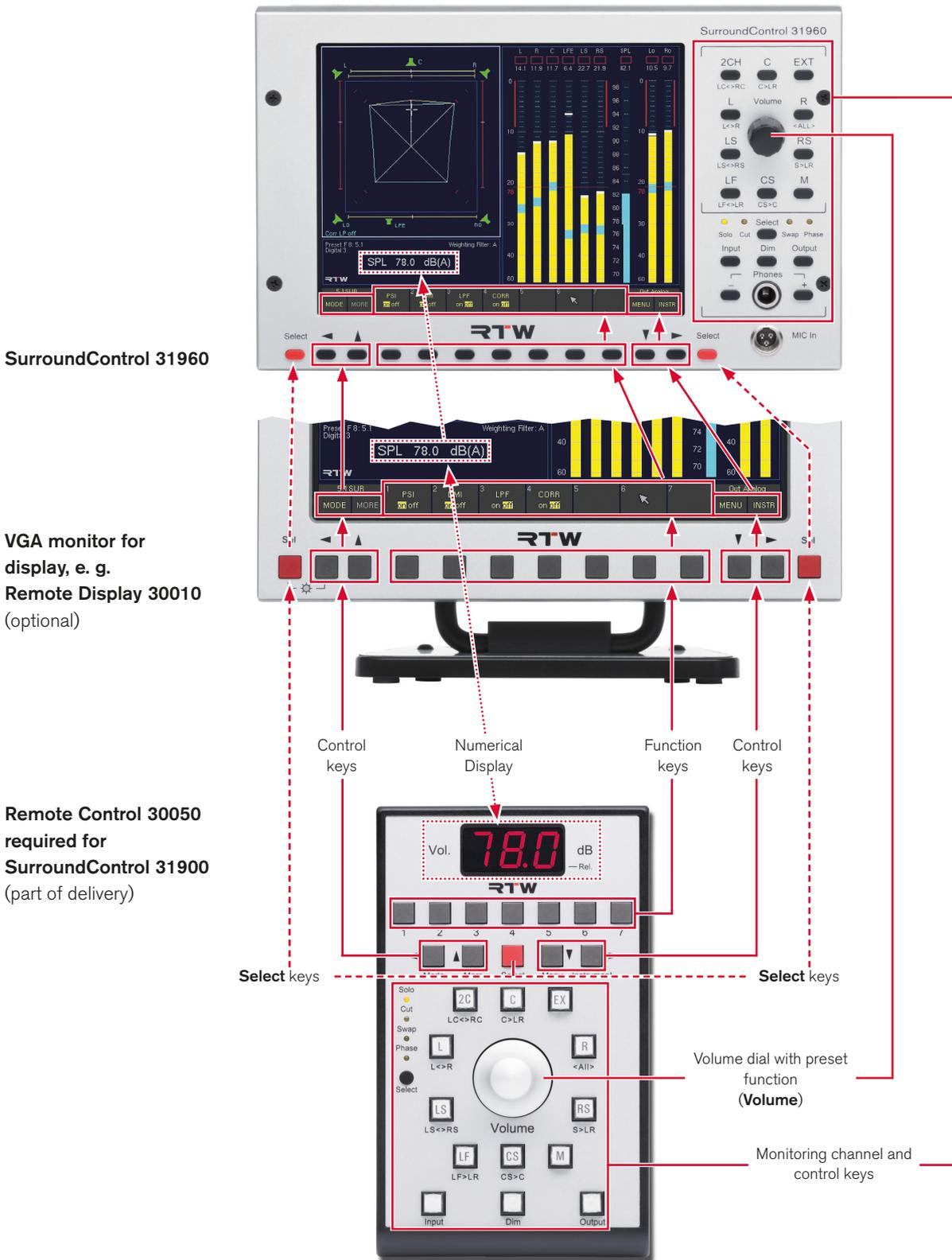
Besides controlling the metering functions, the Remote Control 30050 for the 31900 series and the control panel of the 31960 series are fully featured monitoring controller units with loudspeaker channel keys, several channel functions such as Solo, Cut, Swap and Phase reverse, numerical readout of the volume level set, input and output selection, and DIM or MUTE function. Up to three Remote Control 30050 units can be connected to the 31900 series (31960 series: up to two units).
