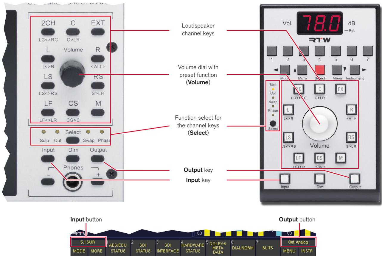
On top of controlling the SurroundControl's metering functions, the Remote Control 30050 as well as the 31960 Series control panel are also fully featured surround monitoring controllers with numerical readout of the volume level set.
