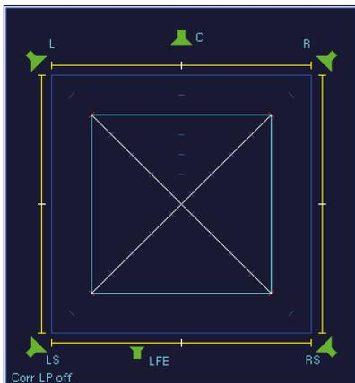
1 | Incoherent noise with same levels in the channels L, R, LS and RS, set to the reference monitoring sound pressure level. In each case the correlation is  $r = 0$ , phantom sound sources are not locatable.
