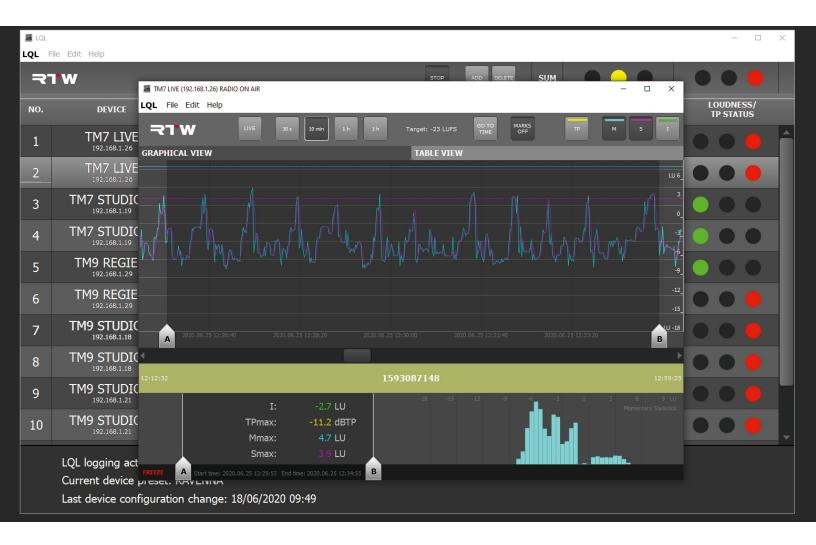
With the **LQL - Loudness Quality Logger**, RTW offers a logging console that collects data via network from various TouchMonitor devices with activated Loudness and Logging Data Server licenses in order to provide an offline storage capability that goes along with some add on features.
