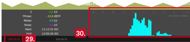
**NOTE** - A reason for missing data may be the overflow of TouchMonitor's data cache (3 hours). Data from the beginning of the measurement may have fallen out, so the start event gets lost. Please take care to connect the LQL with TouchMonitor just in time to assure the complete aquirement of the cached data. The evaluation resp. the real time collection of data will temporary pause until the cache is empty.
