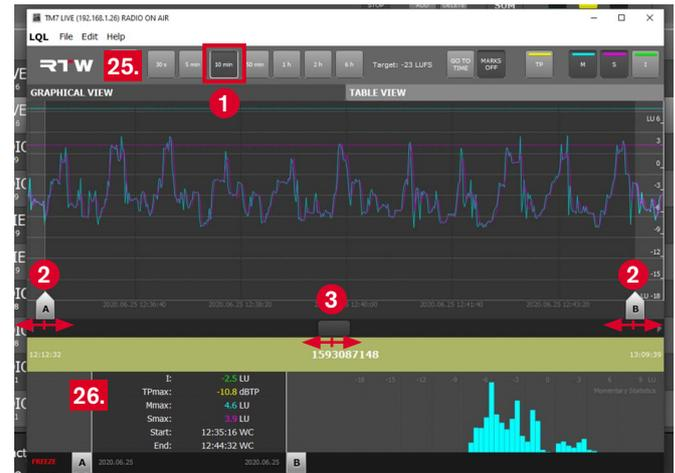
26. Repeat these steps until the markers are on the exact positions you need. The numerical display shows the recalculated values for the selected span.
