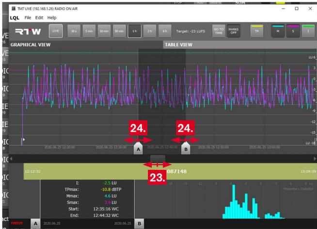
24. Click and hold the left mouse key to move the markers and to place them around the span you want to evaluate. While moving the markers LQL will recalculate the numerical readings on the fly and read the new start and stop time.
