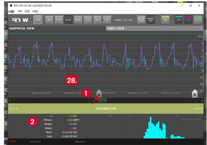
29. If for example the start time being displayed below the numerical section turns to red, it is possible that LQL didn't get a biunique start event. This causes incorrect measuring results because of missing data.
