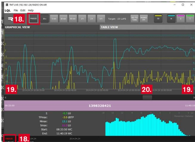
19. Use the arrow buttons on the left and on the right below the graph to move back and forward in steps according to the selected scaling factor.
