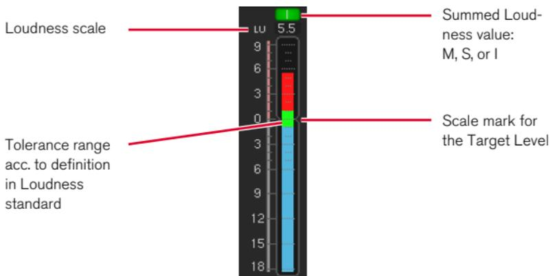
The **Loudness Bar** instrument shows the combined total loudness consisting of the summed single channels of a signal. This instrument shows a bargraph representing one of the three available measurements with different integration time constants. For stereo sources, the L and R channels are summed. For 5.1 sources, the five main channels (5.0) are used for the measurement.
