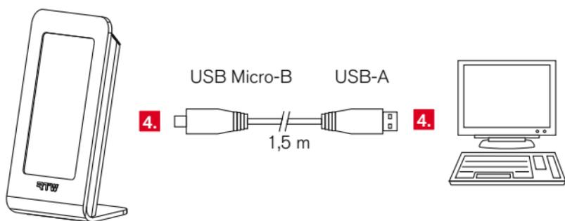
4. If not proceeded yet, connect TM3-Primus to a computer with internet connection using the delivered USB connecting cable.
