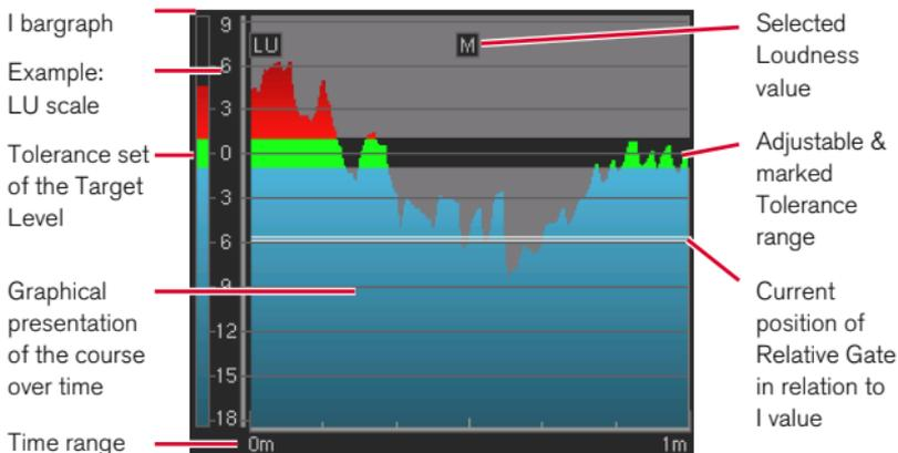
The Loudness **Chart** instrument displays the progress of a measurement (TP, M, S, or I value over time) as line or colored area under curve on a coordinate system with selectable time range. Additionally, the tolerance range can be displayed as a kind of corridor. A dynamic line shows the position of the Relative Gate in relation to the I value, and an additional bargraph for the display of the current I loudness value can be selected.
