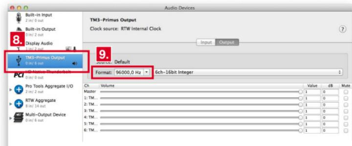
Check sample rate (Format) and adapt, if necessary
