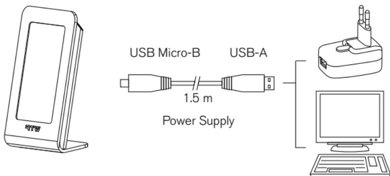
Power supply is provided via USB 2.0 Micro-B connector on the rear side of the unit, either using the delivered USB mains adapter or directly from a computer. The delivered USB connecting cable shall be used.
