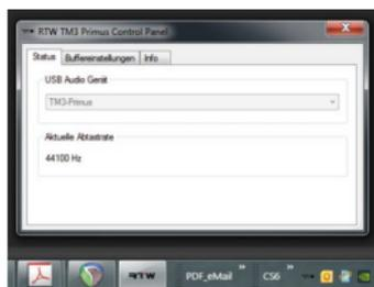
4. If not done yet, install the **RTW Primus Audio Driver** including the **RTW TM3 Primus Control Panel** on Windows® systems as described in **Use of USB Audio Signals** section of chapter 2 | **Installation**.
