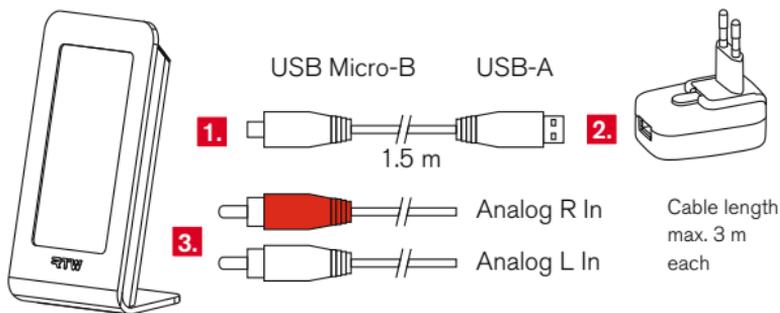
1. Plug the Micro-B connector of the delivered USB connecting cable to the USB Micro-B connector of the unit.
