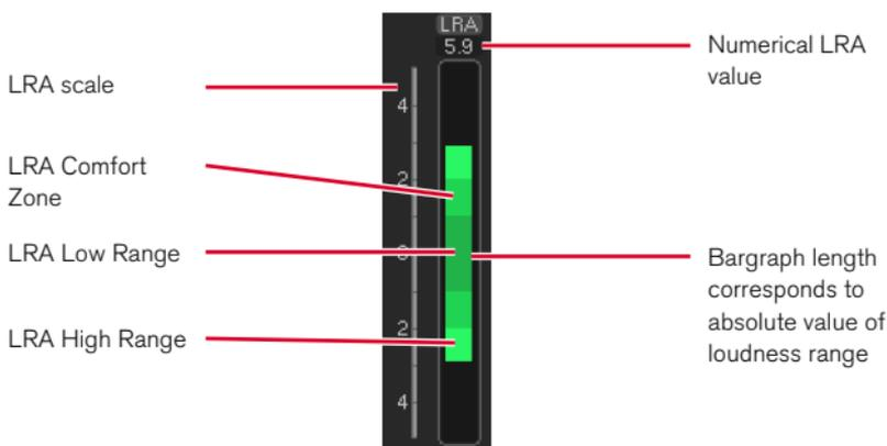
The **Magic LRA** instrument provides a graphical representation of the Loudness Range (LRA) descriptor. LRA is a statistical method used to measure the variation of loudness across an entire program, where lower LRA values represent lower program dynamics. In this way, the LRA measurement can show whether a program has a continuously constant loudness (low LRA values) or a high variation between low and high level components (high LRA values).
