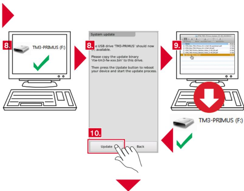
8. TM3-Primus will be recognized by the computer system as a USB drive (**TM3-PRIMUS**). As soon as the unit has been detected, the **System update** menu page appears displaying notes about how to proceed.
