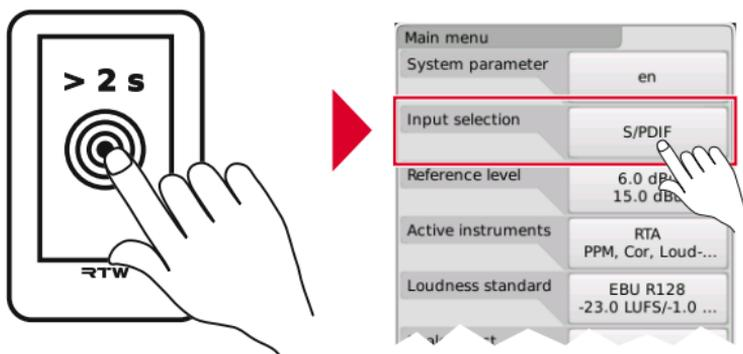
Selecting the active signal input for the current measurement is namely done by answering the initial request for the domain, but when touching and holding the screen for more than 2 seconds you can change the input with the **Input selection** option of the setup menu. In this way, switching between several sources connected to the unit is done very easily.
