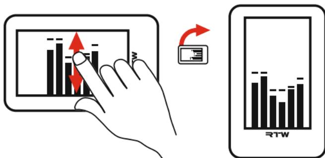
1. During normal operation wipe across the touchscreen with your finger in vertical direction of the lying unit. The display changes from horizontal to vertical orientation.
