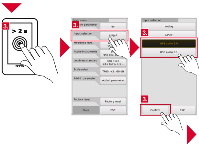
3. Access the menu, touch **Input selection** and select **USB audio 2.0** or **USB audio 5.1** according to the channel count of the audio signals to be measured. **Confirm** and **Store** the settings.
