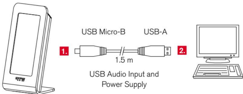
1. Plug the Micro-B connector of the delivered USB connecting cable to the USB Micro-B connector of the unit.
