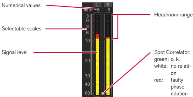
The **TP/PPM Bargraph** instrument provides a vertical bargraph display for the individual channels of the active signal source. The signal level is displayed for each channel. Using the TP/PPM, please ensure that the levels of the individual channels correspond to the requirements defined for the audio program measured.
