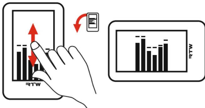
1. During normal operation wipe across the touchscreen with your finger in vertical direction of the upright standing unit. The display changes from vertical to horizontal orientation.
