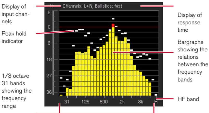
The **RTA** instrument displays the spectral content of the input channels using 31 filter bands in 1/3 octave steps. It measures the magnitude of an input signal per frequency band. An optional "H" band shows spectral signal components above 20 kHz. The display's reference point and resolution can be shifted for a clearer readout in the window. The RTA level display is always relative.
