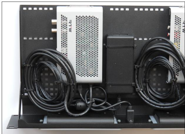
16. Connect the external power supply to mains supply. The device will initiate its system startup sequence. After the boot-up the unit is ready for use.
