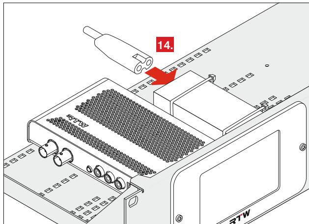
14. Finally, connect the mains cable to the power supply but not yet to mains supply.
