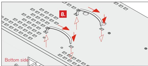
8. Take two cable ties and pass them from above through the both rectangular holes located in a distance of 6 cm from the smooth rear side of the interface box. On the bottom side, move them in parallel to the front side of the frame to the rectangular holes located nearby the interface box. Pass the cable ties through these holes back to the upper side of the frame.
