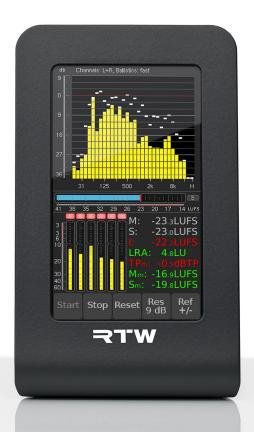
Touch screen layout • views selectable just by finger wipe • Stereo inputs: analog, SPDIF, USB • Surround audio via USB digital output • Loudness according to all relevant standards • PPM/True Peak or VU • Chart • RTA • Audio Vectorscope
