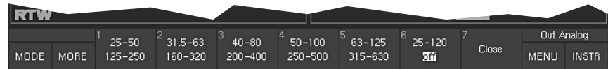
Fig. 5-38: Second Toolbar function layer of the LF test signal (displayed after selecting MORE)
