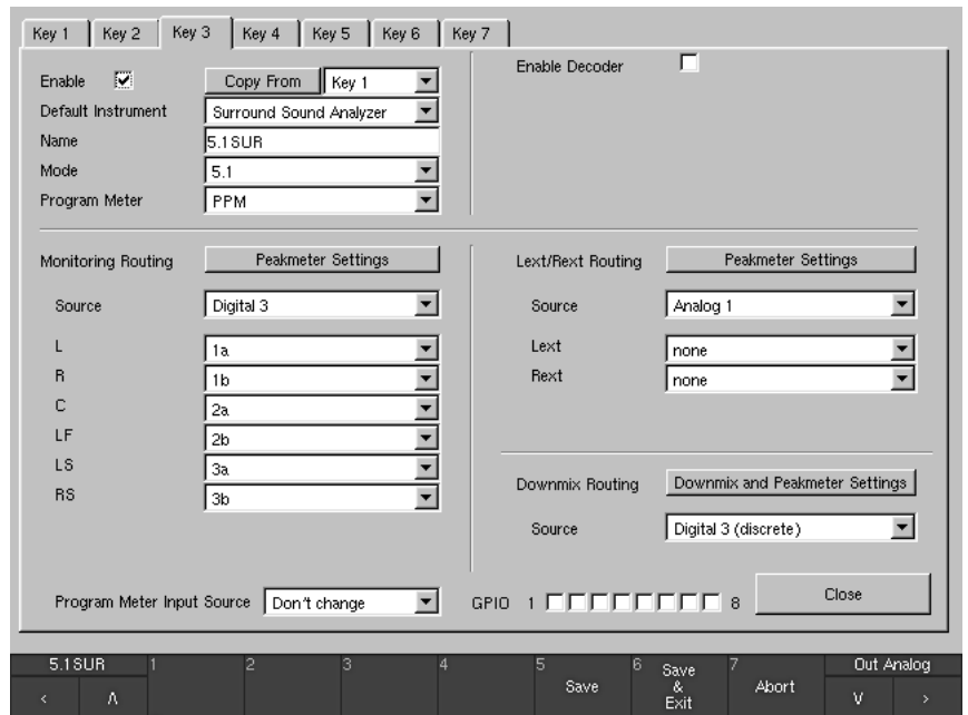
Fig. 3-12: The Key 1 to 7 Sub Preset menu tabs of the Monitoring Input Routing setting
