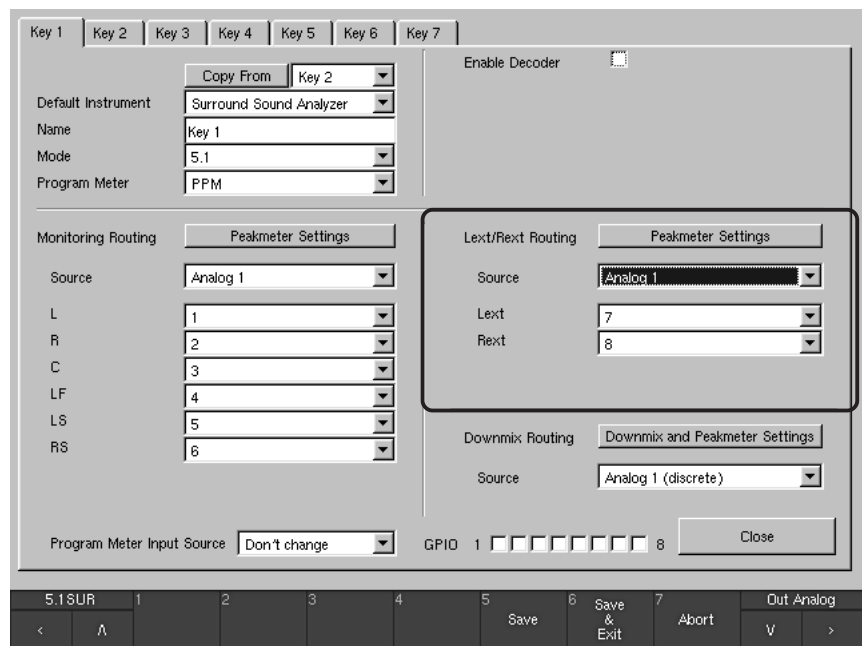
Fig. 6-32: The Lext/Rext Routing section
