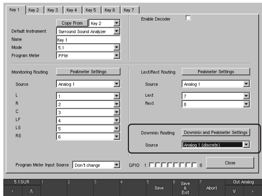
Fig. 6-33: The Downmix Routing section
