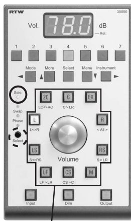
Channel keys on the Remote Control 30050: L is solo Also see Figs. 4-2 and 4-3
