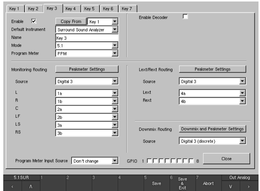
Fig. 6-17: The Key 1 to 7 menu tabs after pressing the Monitoring Input Routing button (screen content might change depending on the channel format used)
