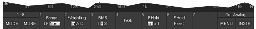
Fig. 5-25: Second Toolbar function layer of the RTA instruments (displayed after selecting MORE) in Multi-Channel mode
