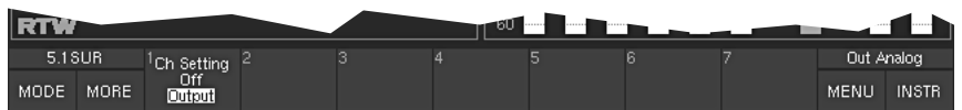
Fig. 5-32: Second Toolbar function layer of the MONITORING instrument (displayed after selecting MORE)
