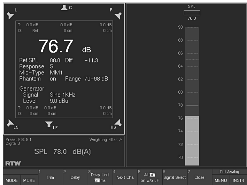
Fig. 2-11: The calibration instruments (CAL) displayed in window 3 (highlighted with a white frame)
