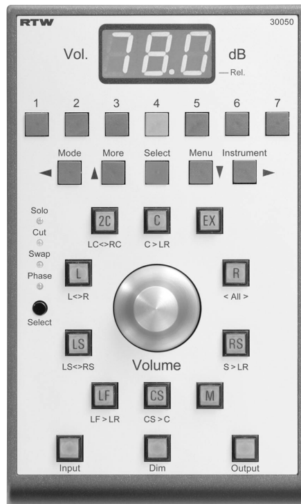
Fig. 2-20: The Remote Control 30050 for function and monitoring control of the 31900 units
