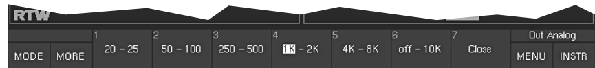
Fig. 5-40: Second Toolbar function layer of the Sine test signal (displayed after selecting MORE)
