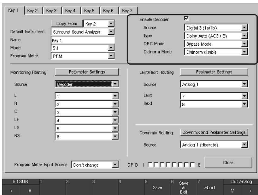
Fig. 6-28: Example for the enabled Dolby® decoder (only with D and SD versions)
