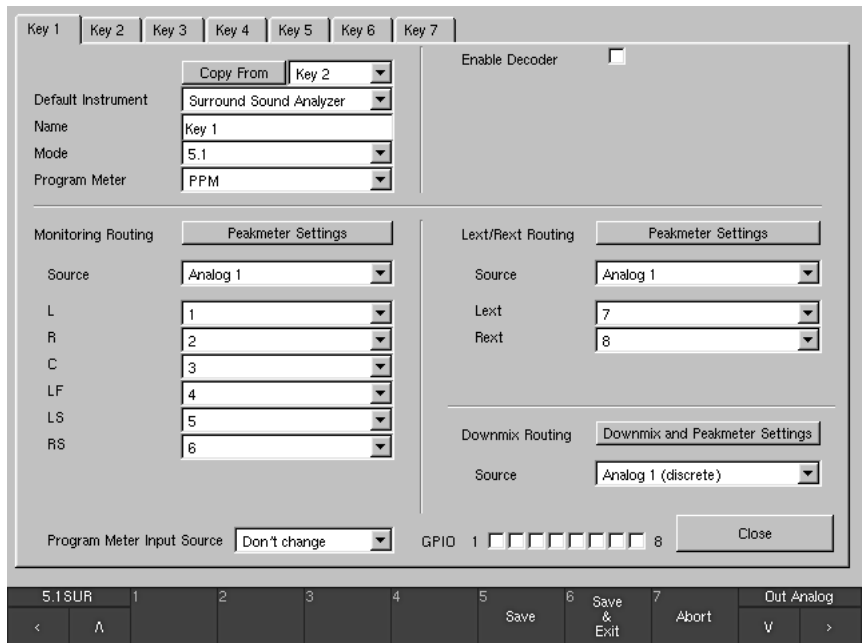
Fig. 6-20: Global Monitoring Input Routing menu page with „5.1“ mode selected
