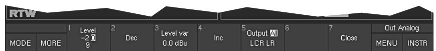
Fig. 5-37: Screen display of the first function layer of the LF-Test signal. Select MORE to display additional functions (level 2)
