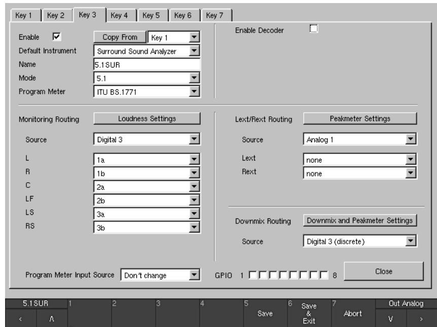
Fig. 3-16: The Key 1 to 7 Sub Preset menu tabs of the Monitoring Input Routing setting with ITU BS.1771 selected for Program Meter
