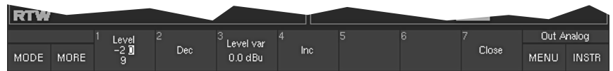
Fig. 5-39: Screen display of the first function layer of the Sine signal. Select MORE to display additional functions (layer 2)
