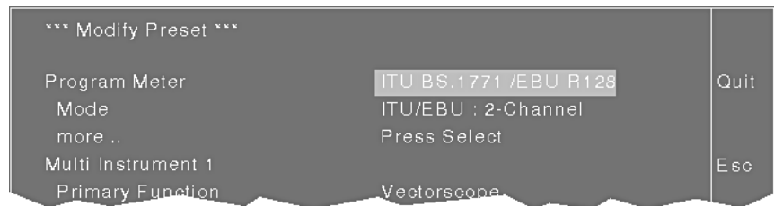
Fig. E 5-7: The Modify Preset menu, when ITU BS.1771/EBU R128 mode is selected
